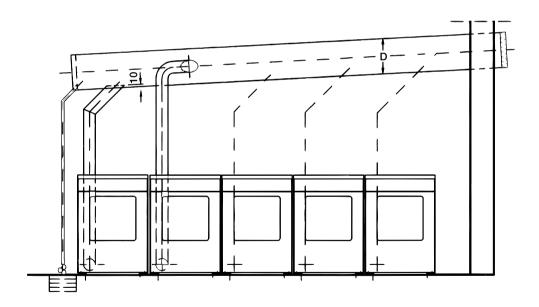
Moist air can be ducted outside by a wall vent kit or window vent kit, both of which are available from the Miele Spare Parts Department.
